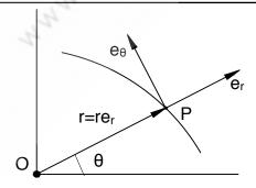
$$V = (\dot{r}) e_r + (r\dot{\theta}) e_\theta = (V_r) e_r + (r\omega) e_\theta = (V_r) e_r + (V_\theta) e_\theta$$
